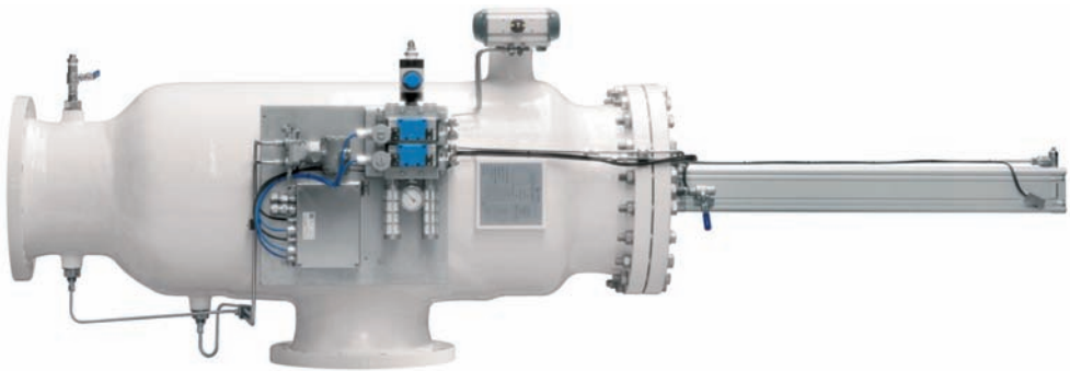
Fig. 5: Installed and ready for operation, e.g. 16" unit/400 mm nominal diameter for a capacity of 1800 m 3 /h (EExd design). Can be installed in any position in the piping system. The units is in operation in a seawater system for QAFCO in Qatar.
