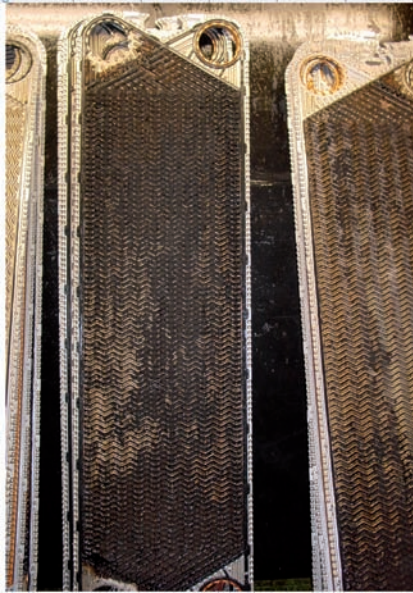
Fig. 4: Plate heat exchanger with blocked surface
