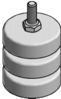
A technical drawing of a magnetic insert. It consists of a cylindrical body with three distinct horizontal sections. On top, there is a hexagonal nut with a threaded rod protruding from its center. |
